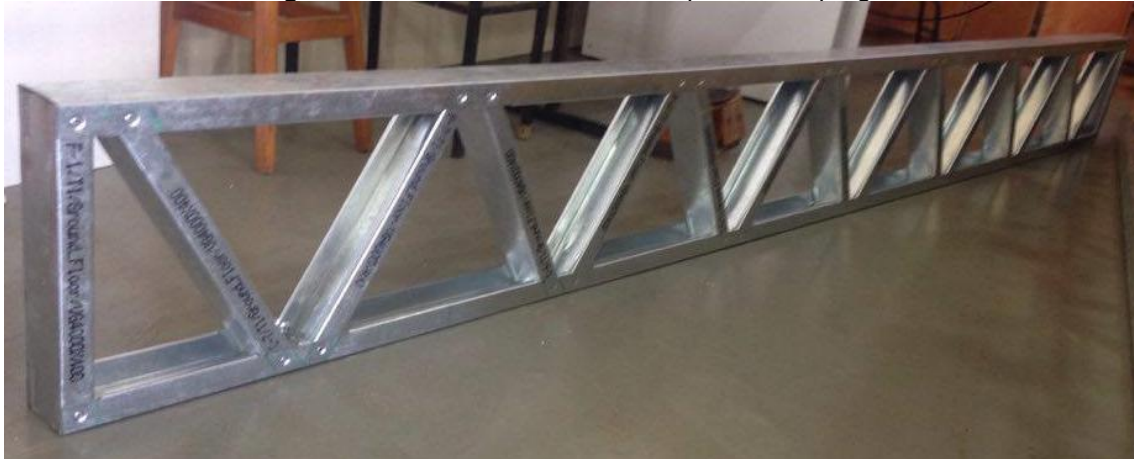
Figure 1: Beam truss used in the experimental program.
