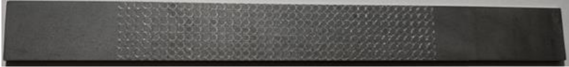
Figure 3: Mesh of circles with d_0 of 2.5 mm on the surface of the test specimens.
